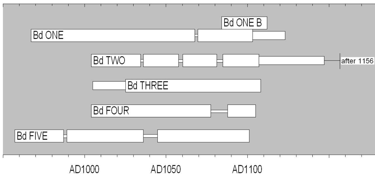
**Figure 8:** Bar diagram showing the relative positions of overlap of the dated sections of ring-width series from the five boards of the Buttsbury door. The thinnest bars represent missing rings and the slightly thicker bars represent additional rings present on the board but not incorporated in the cores extracted.
