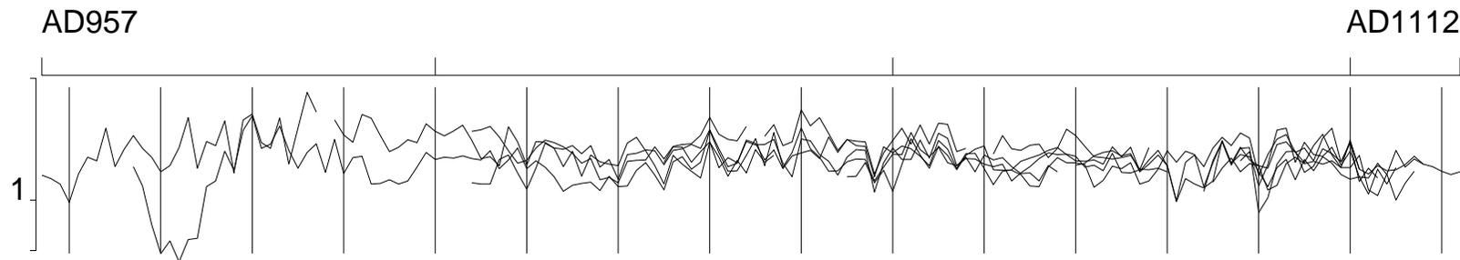
**Figure 7:** The final set of overlapping curves from measured sections of the 5 boards. The *x*-axis is in relative years, the *y*-axis is a logarithmic scale of ring width in mm.
