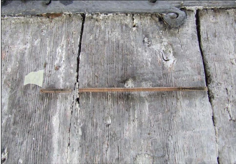
**Figure 4:** Photograph showing the core for board 3 (right) along with the additional section of core from board 2 from the overlapping part of the board. The masking tape right-hand edge marks the end of the core for board 2 taken from left to right.
