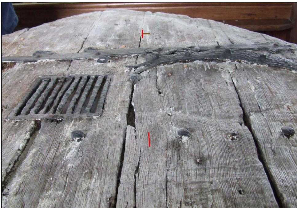
**Figure 5:** Photograph showing the approximate position of the additional part of board 2 from the overlap (brown line), with the red lines indicating how the grain drifts down the length of the board, necessitating the addition of rings to the last measured ring from the coring position to judge the last ring of the board itself.
