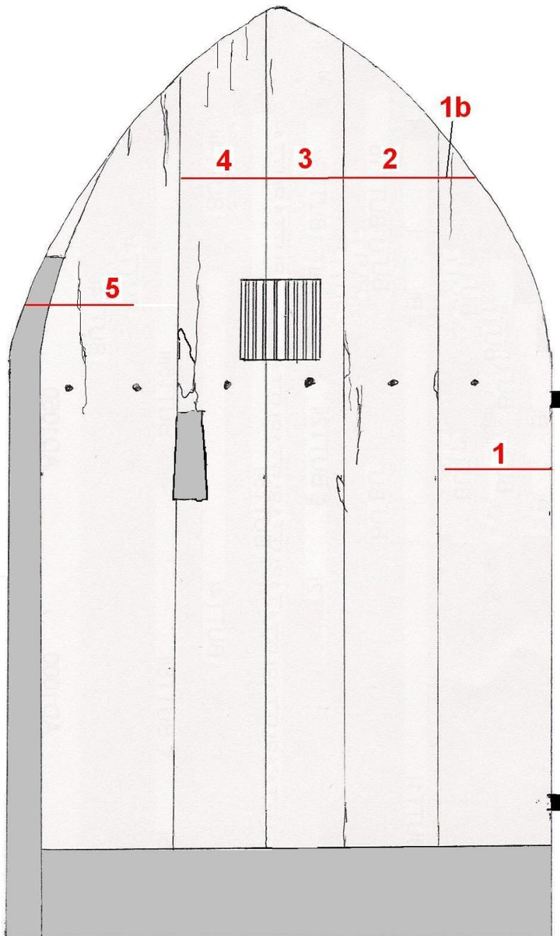
**Figure 3:** Sketch of the front of the door showing the approximate positions of cores removed. Dark grey areas represent newer wood additions.
