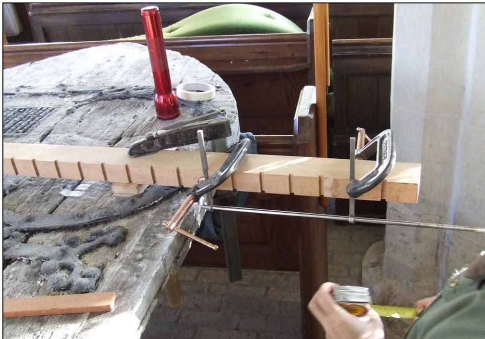
**Figure 2:** Coring of the boards using the micro-borer
